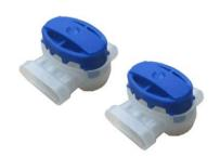
IDC Connectors feature a sharp internal metal insert that safely penetrates wire insulation with a simple pressing motion. Once it is locked in place, the connector securely holds the wires in place, creating a quick and easy wire connection. These connectors are particularly useful for automotive accessories, marine connections and lighting applications.
